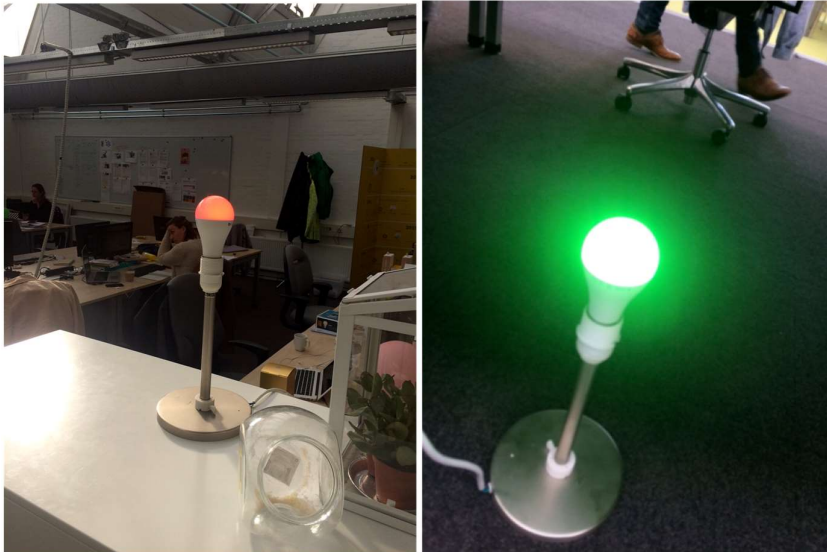
Figure 4: Example of the smart light bulb when tariffs are high (left) and when tariffs are low (right)
